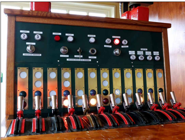
The Westinghouse 'L' frame, rescued and restored, is now fitted to the signalbox and ready for business at the start of its second career.
