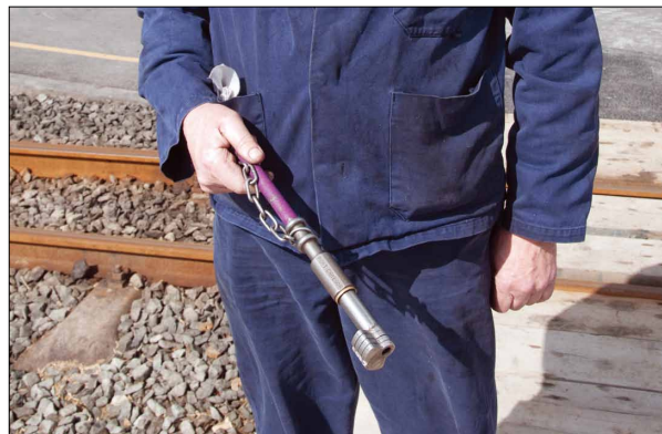
This is a Pont Croesor - Beddgelert token obtained from the cabinet after permission from Control. There's only one, so it's quite safe, though trains may enter the section with a 'ticket' - ask Google.
