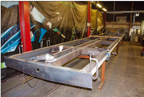
Boston Lodge will turn out underframes for cars of all different sizes and gauges if you give them a drawing - and a bit of cash.
